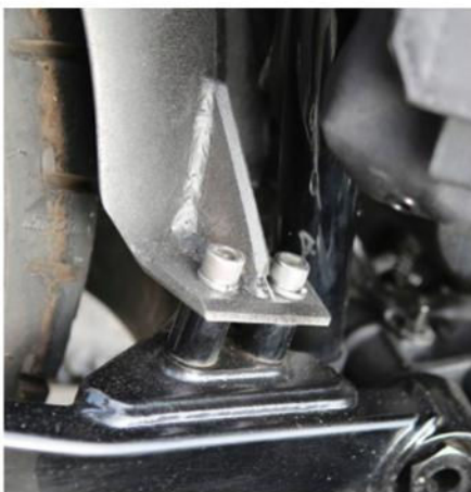
Attention to detail — clever way to mount the rear fender to the swingarm.
