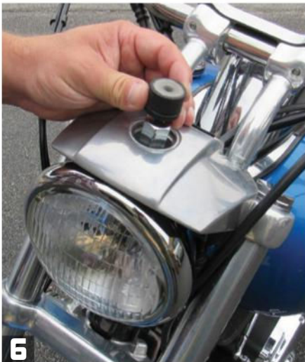
6 After properly positioning the headlight as per the accompanying sidebar and tightening the hex nut using a 3/4" socket, install the kit's rubber mount onto the hex nut and tighten it.
