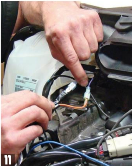
11 Connect the orange wire from the Big Bike harness to the purple 12-volt accessory wire and the two LED light ground wires, and the green Big Bike harness wire to the bike's black wire.
