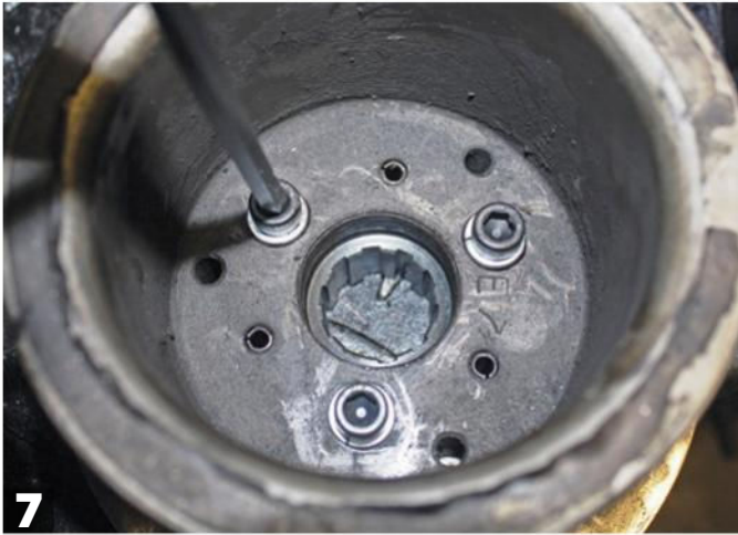
10 The new sprocket insert has three split pins for alignment. Press them into the insert, and then place the insert in the front pulley.
