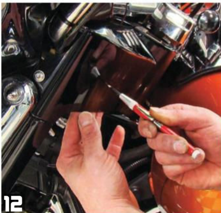
12 Use a pin punch to locate a spot for the switch and dimple the panel to be drilled.
