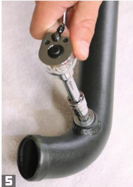
5 Using a light coating of anti-seize and a 10mm Allen, screw one of the supplied sensor plugs into the top location on the forward header.
