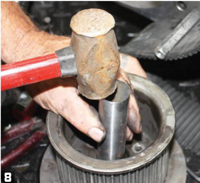
8 The insert comes out easily with a few light taps.
