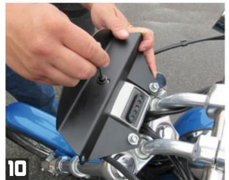
10 Loosely install one of the kit's black screws and flat washers into the slot and rubber isolating mount using a 5/32" Allen. You'll tighten this bolt to 40 in.-lbs. in Step 12.
