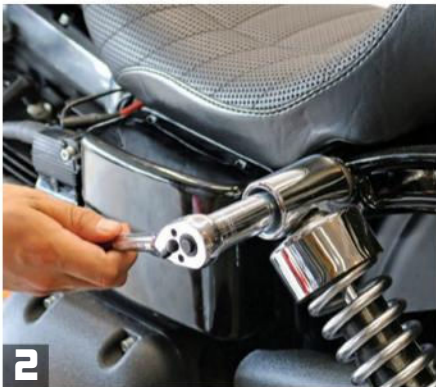
2 Remove the top shock mounts with a 3/4" socket. It requires some force to loosen.
