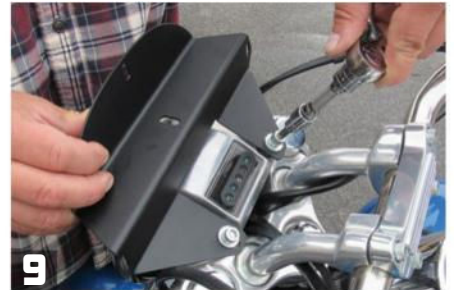
9 With a little blue Loctite on the bolt, install the mount onto the front end using a 1/4" Allen but leave the bolts loose for now. You'll tighten these bolts to 12-15 ft.-lbs. in Step 12.
