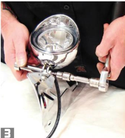
3 Using a 10mm wrench and a 5mm Allen wrench, snug the light pedestal bolt so it doesn't flop around.
