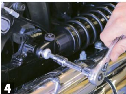
4 With both shocks removed, lower the bike onto the wooden block bringing the wheel up into the fender. Then, after applying red threadlocker to the bolt, loosely install the right-side lower shock bolt using a T50 Torx. Put a supplied spacer on either side of the shock. Leave it loose enough to swing over the top mount. The shocks should be positioned with the adjuster knob on the bottom, facing rearwards, and the serial number facing in.
