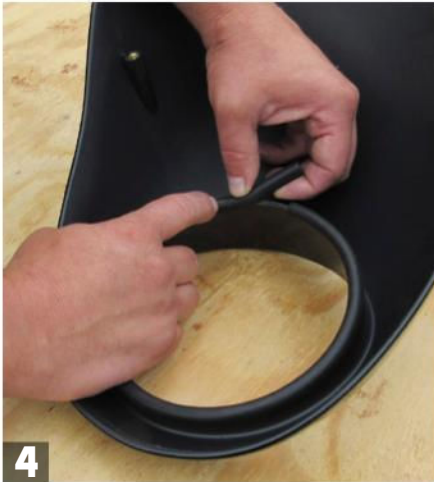
4 Now install the kit's edge gasket around the headlight opening in the café fairing starting at the top and working your way all the way around. The seam should be at the top of the opening.
