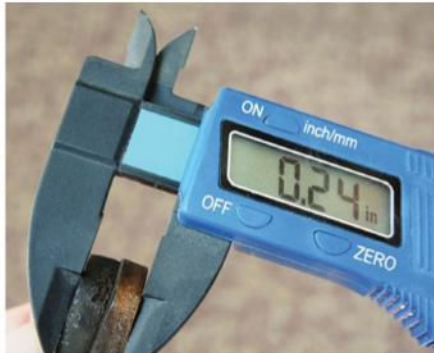
After setting a zero reference, the calipers will do arithmetic for the user when comparing thicknesses.
