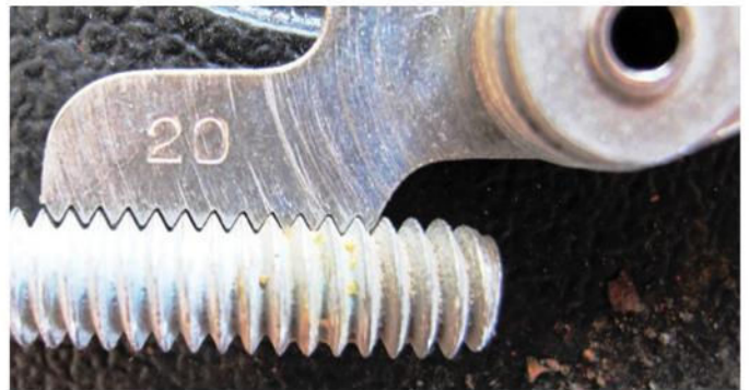
Place the notched side of the blade into the threads you're checking. You've found a match when every notch fits every thread on the bolt or shaft.
