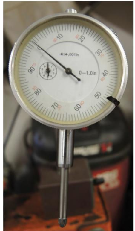
Dial indicators measure movement when the probe at the bottom of the tool is moved towards or away from the dial.
