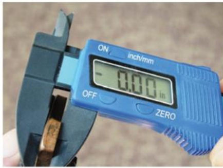
Many digital calipers allow the user to set a zero reference when comparing two thicknesses. This can be helpful if the calipers lack the depth rod.
