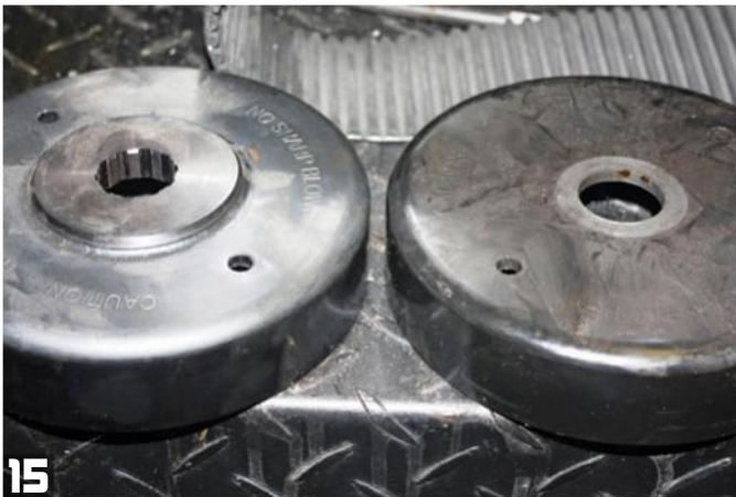
15 The new stator rotor on the left is the heavy-duty one from Twin Power. The stock rotor on the right had a spline length of only .241" and used .260" of washer spacers. This heavy-duty rotor has a spline depth of .500. That is over twice the spline depth of the original rotor for added strength/protection for the splined engine sprocket shaft. Be sure this is clean and has no lubricants on it. Because this rotor has the extra spline thickness, do not use any spacers!
