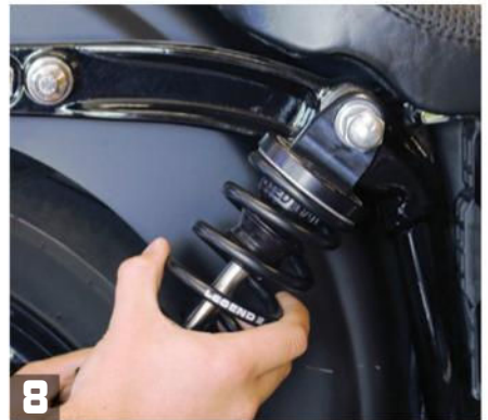
8 To set the sag, simply twist the springs by hand. (the springs are attached to the threaded adjustment collars) Loosen (extend the spring) to increase sag and tighten (compress the spring) to decrease sag. You'll want to have a buddy measure while you sit on your bike with whatever gear you usually wear or carry. Set each side equally.
