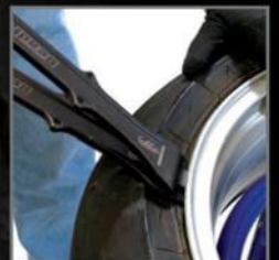
P/N 08-0536 BeadPro FS is designed to easily break the bead on most street motorcycles
