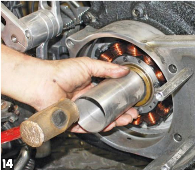
14 Tap the seal in gently and evenly to prevent damage. Never hammer the seal on directly with the hammer head.
