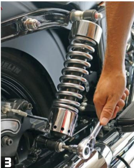
3 Using a T50 Torx on the right and a T50 Torx plus a 3/4" wrench on the left, remove the lower shock mounting hardware and remove the shocks. Be cautious as there still could be some pressure left on the second shock to be removed.
