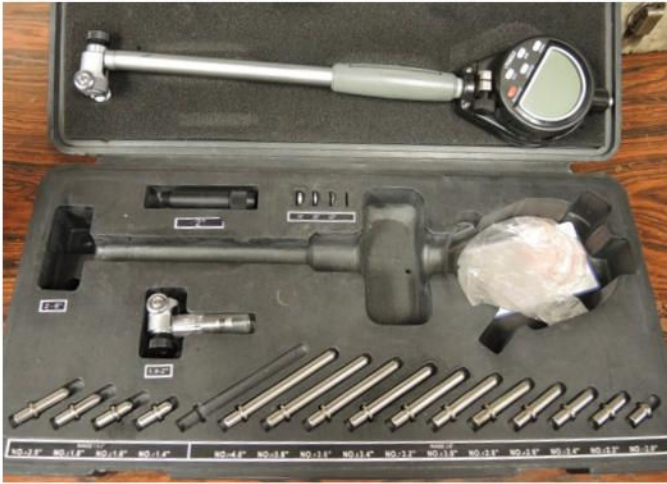
Bore gauges make inside diameter measurements easier and faster than telescoping gauges. However, bore gauges are much more expensive than telescoping gauges.
