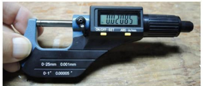
This digital micrometer provides accuracy to .0005" and can switch to metric measurements with the press of a button.
