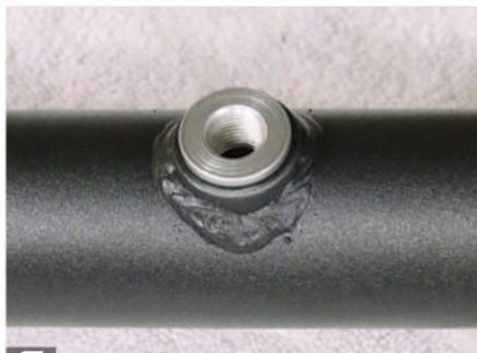
6 Using a light coating of anti-seize, screw in the supplied O 2 adaptors to the remaining two locations.
