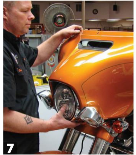
7 Remove the fairing outer shell with a T27 Torx wrench. A total of seven bolts hold it on. Four bolts are on the backside (fairing inner) and three on the windscreen. Disconnect the two headlight connectors to completely remove the outer fairing.
