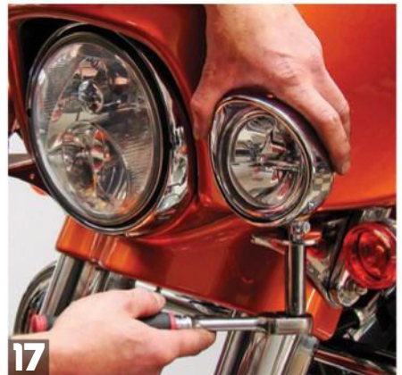
17 Reassemble the front fairing and make final aiming adjustments to the lights and tighten them in place using a 10mm wrench and 5mm Allen wrench for the pivot and a 13mm wrench for the base.
