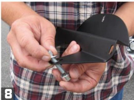
8 Then slip one of the kit's flat washers onto one of the long bolts and put the bolt through the visor (fairing) mount bracket as shown. Then slip one of the kit's 1/2"-thick spacers over the bolt and under the mount.
