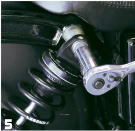
5 Now raise the bike up until the upper shock mounting hole can easily slide onto the stock stud. Slip a washer over the stud, followed by the shock, another washer, and then a spacer. Apply red threadlocker before reinstalling the stock nut with a 3/4" socket.
