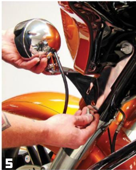
5 Mount the new driving lights to the bike using a 9/16" deep socket and route the wires to under the fairing.
