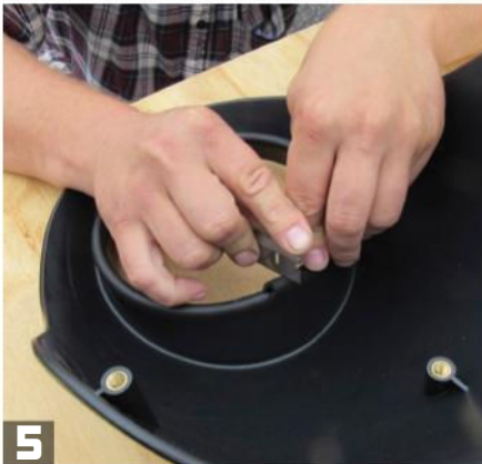
5 Our edge gasket is a little too long, so we have to cut about 1/2" from the end of the edge gasket using a razor blade.
