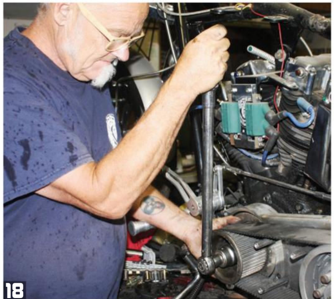
18 Tighten it up using a torque wrench; tighten the nut to 150 ft-lbs. This is very important because this is what holds everything in place and allows no movement of the spline areas. Any movement over time with the splines on the rotor or the sprocket insert will cause damage and fail again. Take your time and do it correctly the first time! AIG
