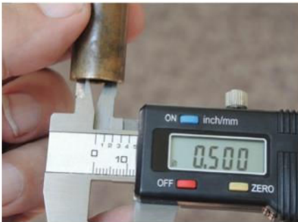
Use the upper jaws when making inside measurements with a caliper.
