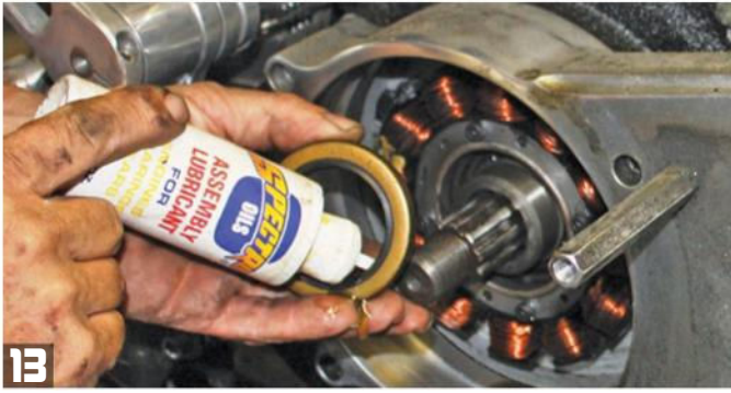
13 Time to install the new engine sprocket shaft seal. Lubricate the seal lip. Clean the area of the engine case where the seal goes in and apply a very light coating of gasket seal on the seal, not the case. This way any excess will not be pushed into the bearing area.
