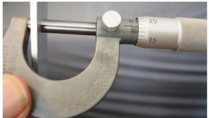
Using a traditional micrometer involves adding the reading from the thimble scale to the reading on the main scale to obtain measurements accurate to .001".
