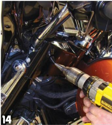
14 Then use a stepped drill bit to open up the hole to 13/16" diameter.
