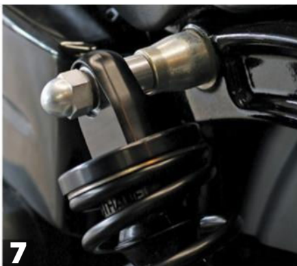
7 For the top left mounting point, with the Legend spacer and shock already slipped on, slide a Legend washer and the stock washer over the stud, followed by some red threadlocker and the stock acorn nut. Tighten it down. For 2008 and later models, slip a supplied spacer on the stock upper left stud. Slide the shock onto the upper stud.
