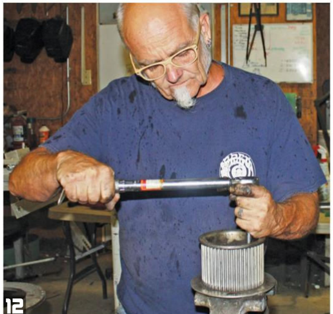
11 Be sure to use the lock washers and the new screws that come with the insert, and for added protection, place some Loctite on the threads.
