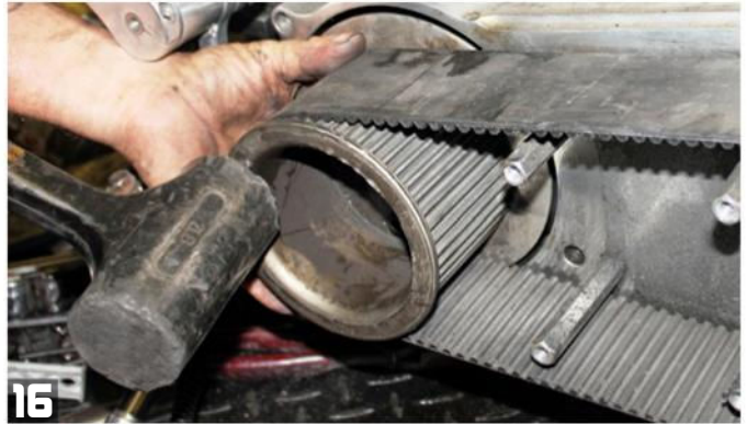
16 Place the primary belt on the front pulley; the unit should go on easily. Sometimes a few light taps with a plastic mallet are needed to be sure it goes on all the way.
