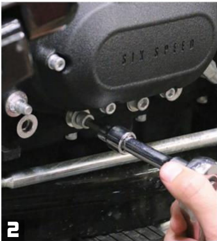
2 The stock exhaust system is removed, and the bike is ready for its new MagnaFlow system. Remove the two bolts underneath the transmission cover using a 1/4" Allen and set them aside for reuse.
