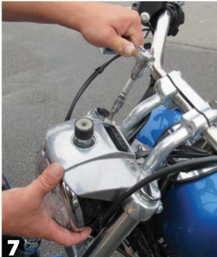
7 Now remove the two bolts that hold the headlight bracket to the front end. Our Dyna's bolts require a 1/4" Allen, but on other models you may need to use a 1/2" socket.
