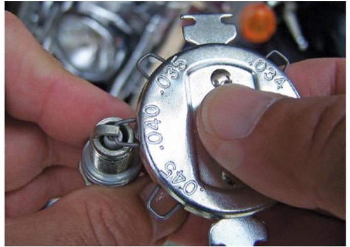
Spark plug gaps should be checked with a spark plug gapping gauge, not a feeler gauge.
