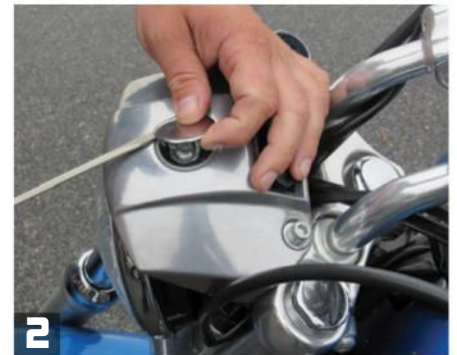
Start by removing the headlight bracket plug that covers the headlight assembly nut using a small flat-bladed screwdriver. This plug will not be reused.
