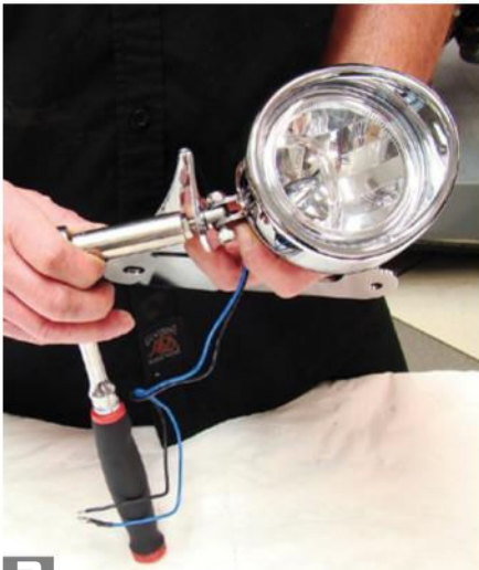
2 Preassemble the lights to the supplied brackets with a 9/16" socket wrench. Do not tighten yet, as light aiming will come later.
