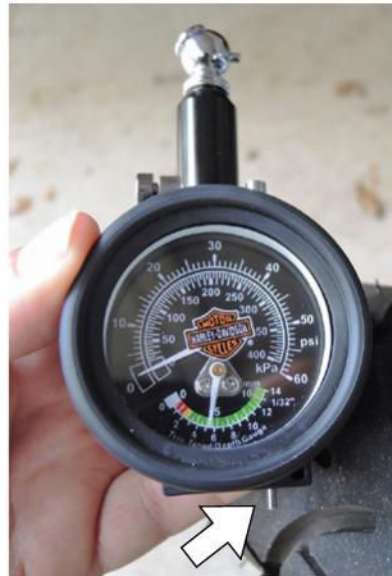
This combination tool from Harley-Davidson measures tire pressure on the large scale and tread depth on the small scale when the depth probe (arrow) is pressed down between tread blocks.
