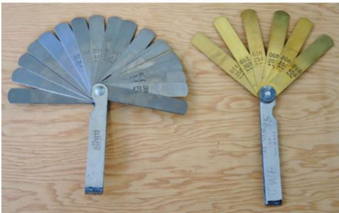
Feeler gauges are available in stainless steel or brass. The brass gauges come in handy when setting air gaps on rotation sensors that contain magnets.
