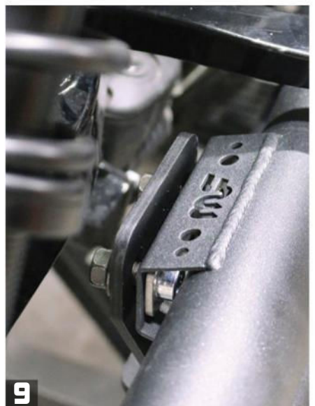
9 Using the supplied bolts and nut plates from MagnaFlow, loosely attach the exhaust system to the mounting bracket using a 3/8" wrench.
