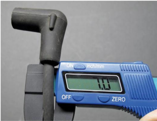
Metric measurements can be made at the push of a button on many digital calipers. I don't know why, but spark plug wire diameters are specified in millimeters.
