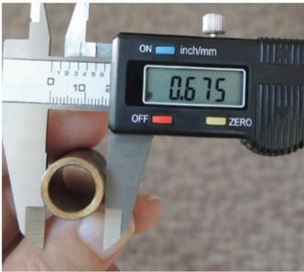
Use the lower jaws on calipers to make outside measurements.
