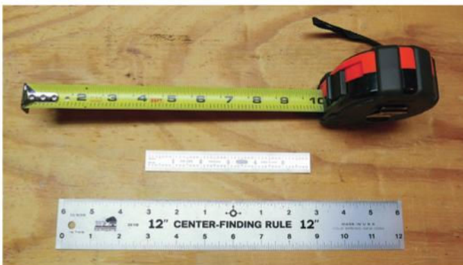
A tape measure and some rulers will suffice for measurements that don't require a great deal of accuracy.
