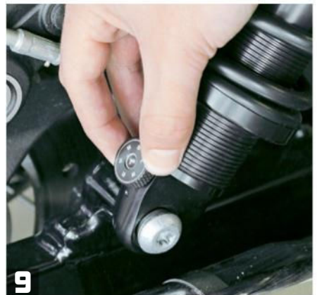
9 Adjust the rebound to your preferred riding style. Start at 3 on both sides and then go up for sport/performance or down for comfort. Set each side equally.
