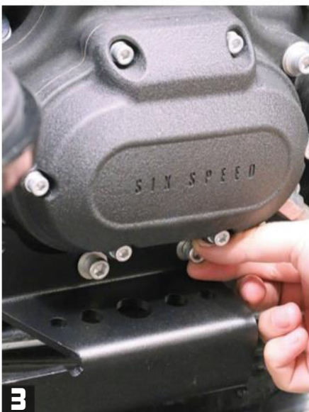
3 After applying some of the supplied red threadlocker to the stock transmission bolts, install the MagnaFlow bracket but leave it hand-tight.
