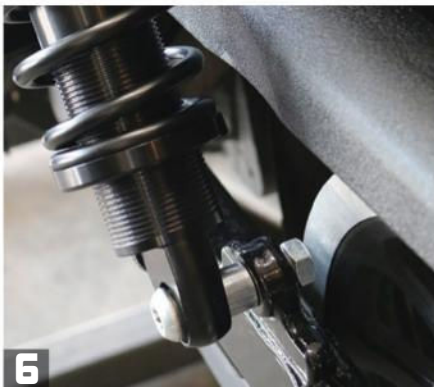
6 After applying red threadlocker to the stock bolt on the lower left shock mount, slide it through a Legend washer, then through the Legend shock, Legend spacer, swingarm bracket, and stock bolt. Be sure to mount the shock with the silver label on the bottom, facing inwards.
