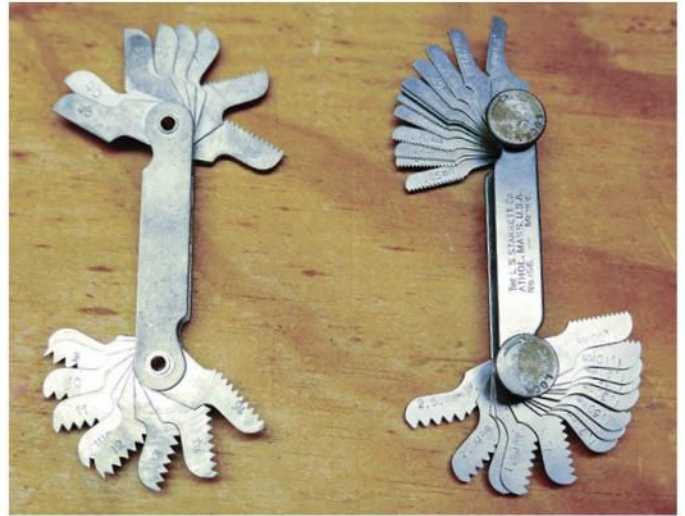
Thread gauges are available for checking thread pitch on metric and fractional bolts or shafts. Using them requires patience and good eyesight, but you'll avoid threading the wrong nut in the wrong place.
