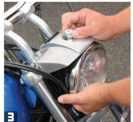
Use a 3/4" socket to remove the nut that holds the headlight assembly to its bracket. Reusing the stock lock washer and beveled washer, loosely install the hex spacer that comes with the fairing kit. The stock nut is not reused.
