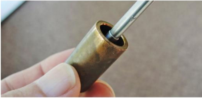
The telescoping gauge is inserted straight into the part being measured, then the measurement is locked in with the gauge's lock screw.
